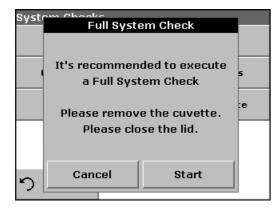
If the instrument detects any deviation relative to the last calibration, a system check has to be carried out.
